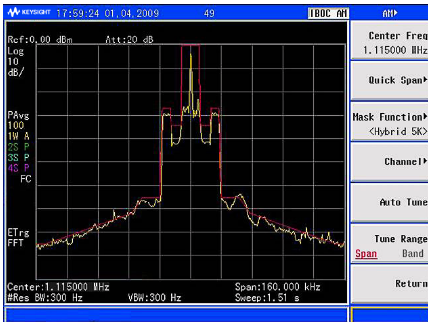
IBOC-AM measurement with N9340B IBC
