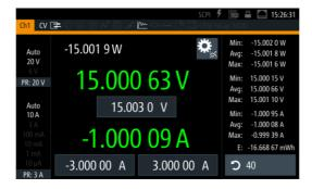
The two-quadrant architecture of this source measure unit allows it to function both as a source and a sink and simulate batteries and loads. The source measure unit automatically switches from source mode to sink mode. As soon as the externally applied voltage exceeds the set nominal voltage, current flows into the instrument. This is indicated by a negative current reading. The linear design of the output stages reduces residual ripple and noise to a minimum.
