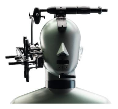
Validated options enable users to perform acoustic measurements of mobile phones in line with standards that are applicable worldwide.
