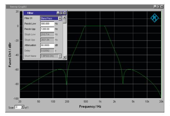
Filters can be programmed simply by entering a few parameters, which takes only a few seconds; they can be used both in the analyzer and the generator.
