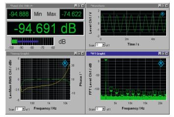
Graphics can be sized with vertical and horizontal cursors; markers and limit traces make evaluation easier. Multiple traces can be superimposed in user-defined colors; background colors, etc., can be selected to meet any requirement.
